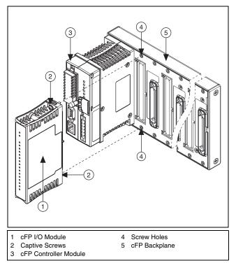
Figure 2. Installing the cFP-DO-403
